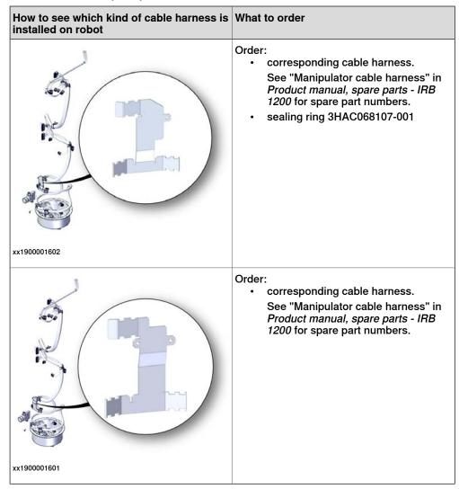
2.4.4 Spare part versions for the housing on Type A robots
